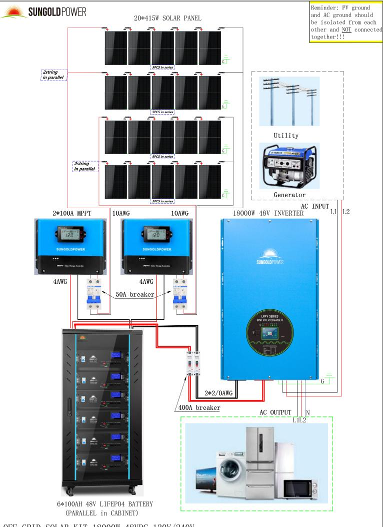
OFF-GRID SOLAR KIT 18000W 48VDC 120V/240V LIFEPO4 20.48KWH LITHIUM BATTERY 20 X 415 WATTS SOLAR PANELS
