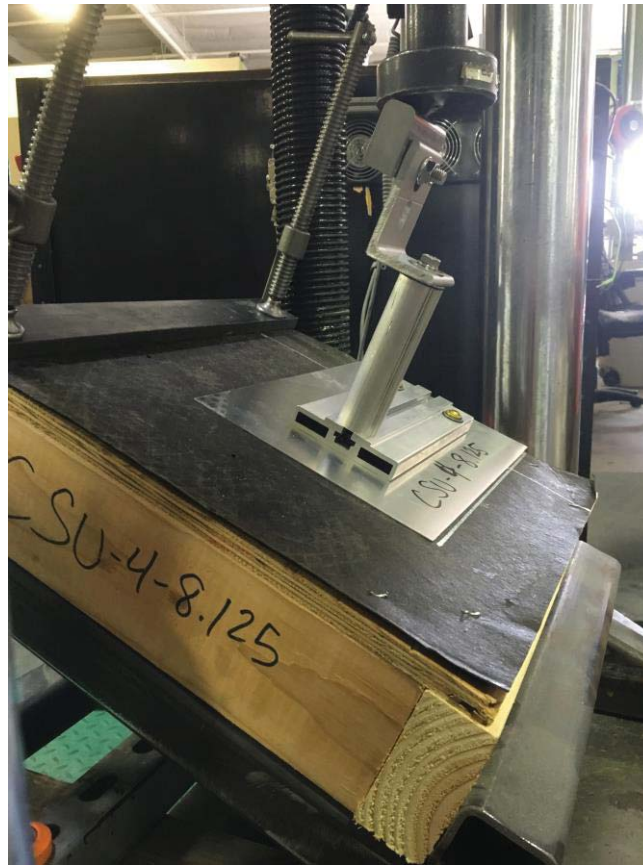
Photo 13: Resultant 6:12 Eccentric Load (Upslope, pre-test)
