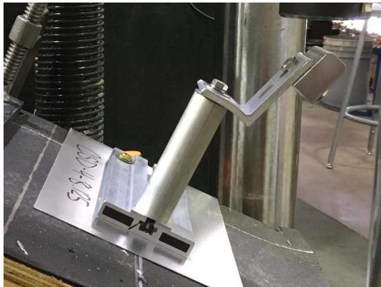
Photo 12: Resultant 6:12 Eccentric Load (Downslope, post-test)
