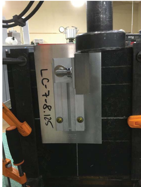
Photo 9: Lateral Perpendicular to Rafter Eccentric Load (pre-test)
