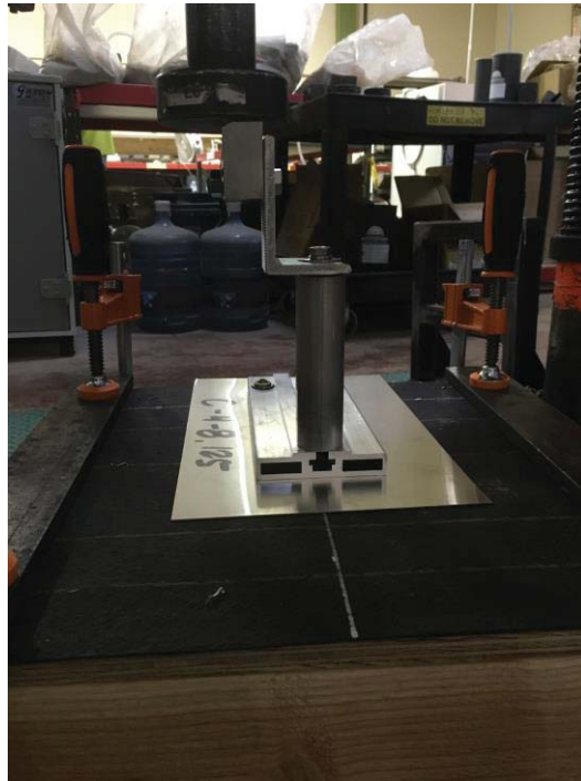
Photo 3: Compression Eccentric Load (pre-test)
