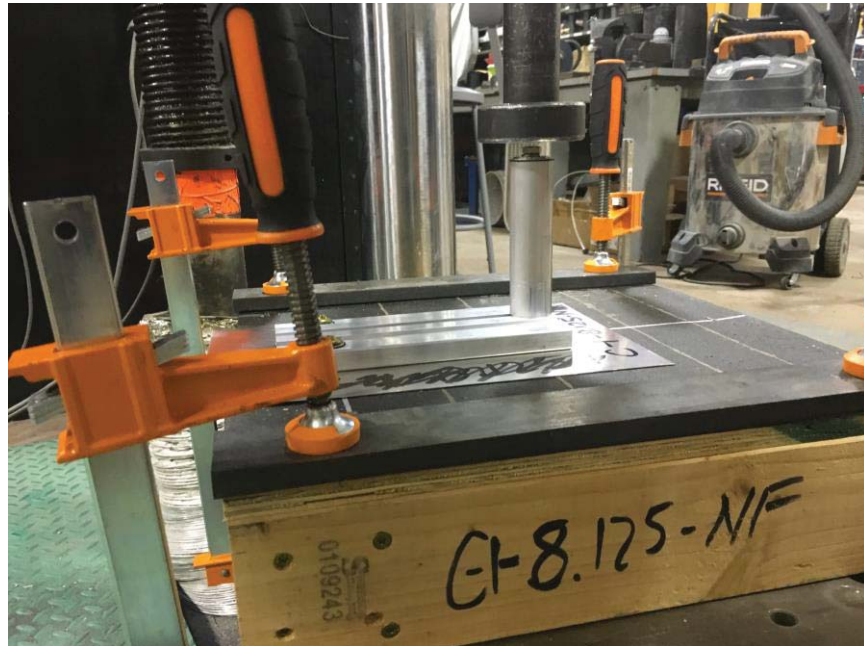
Photo 5: Compressive Eccentric Load (shown without Unirac L-foot, pre-test)
