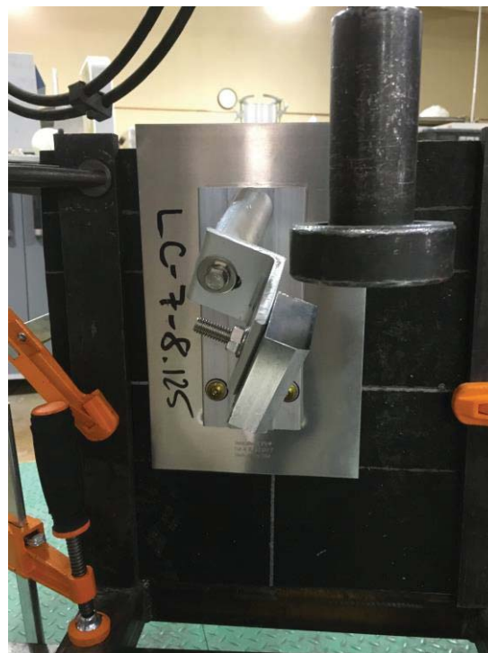
Photo 10: Lateral Perpendicular to Rafter Eccentric Load (post-test)
