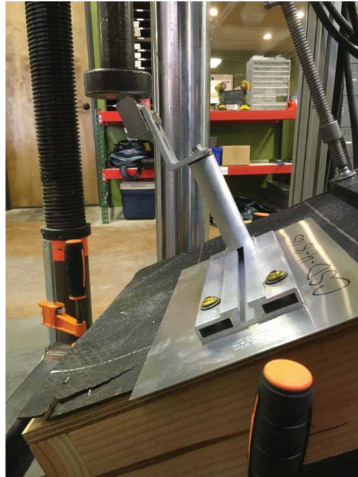
Photo 11: Resultant 6:12 Eccentric Load (Downslope, pre-test)
