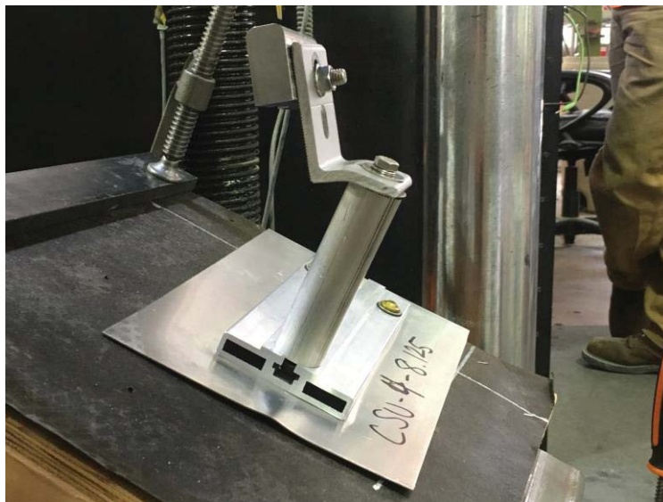
Photo 14: Resultant 6:12 Eccentric Load (Upslope, post-test)
