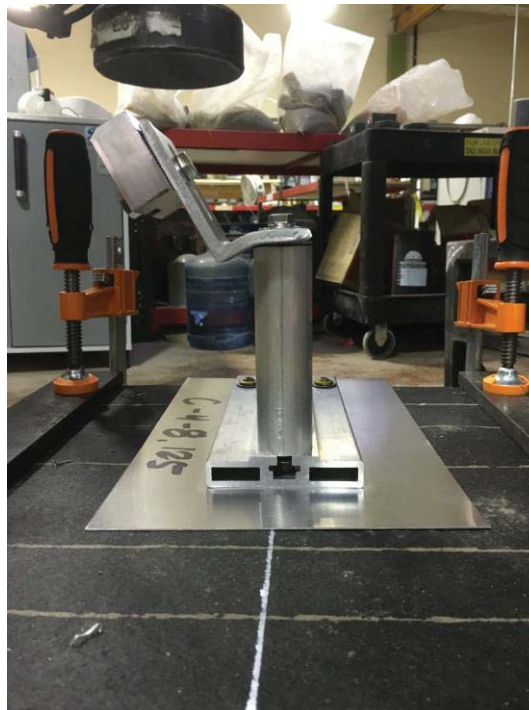
Photo 4: Compression Eccentric Load (post-test)
