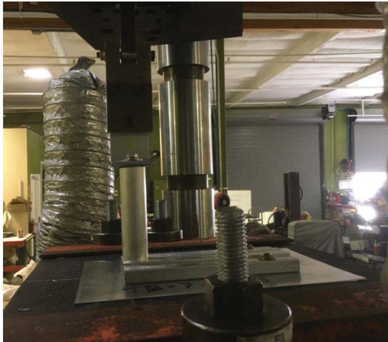
Photo 1: Tensile Eccentric Load (pre-test)
