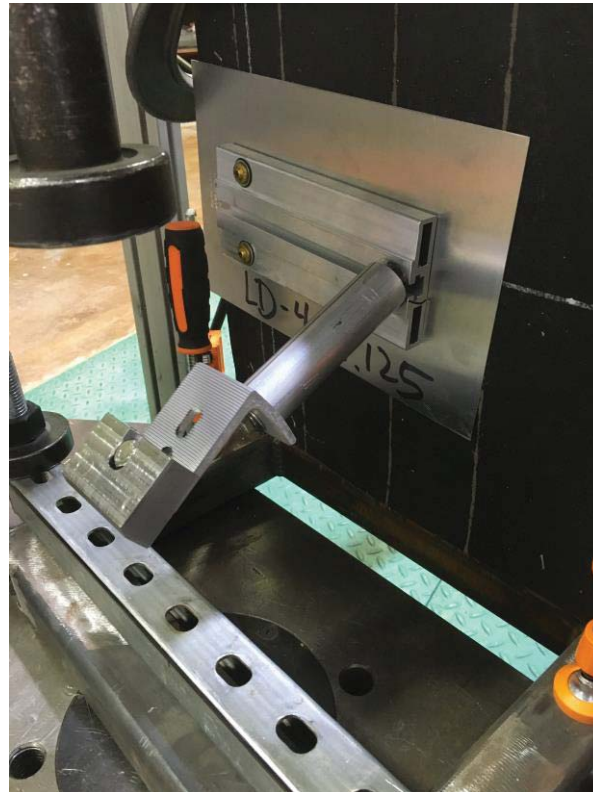
Photo 8: Lateral Parallel to Rafter Eccentric Load (post-test)
