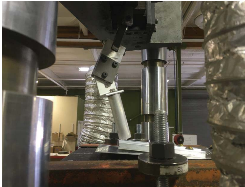
Photo 2: Tensile Eccentric Load (post-test)
