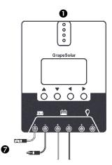
Remove the panel covering. In good sunlight, the charge controller's ● "BAT %" should increase to 100%. When the controller is set to "LOAD ON," the system will provide power through the load control output or through the USB port.
