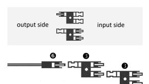
With the other 15-ft MC4 cable **⑤**, connect one branch connector **⑤** with the "male" output to the "female" end of the cable. Connect an additional "male" output branch connector **⑤** to the attached branch connector.
