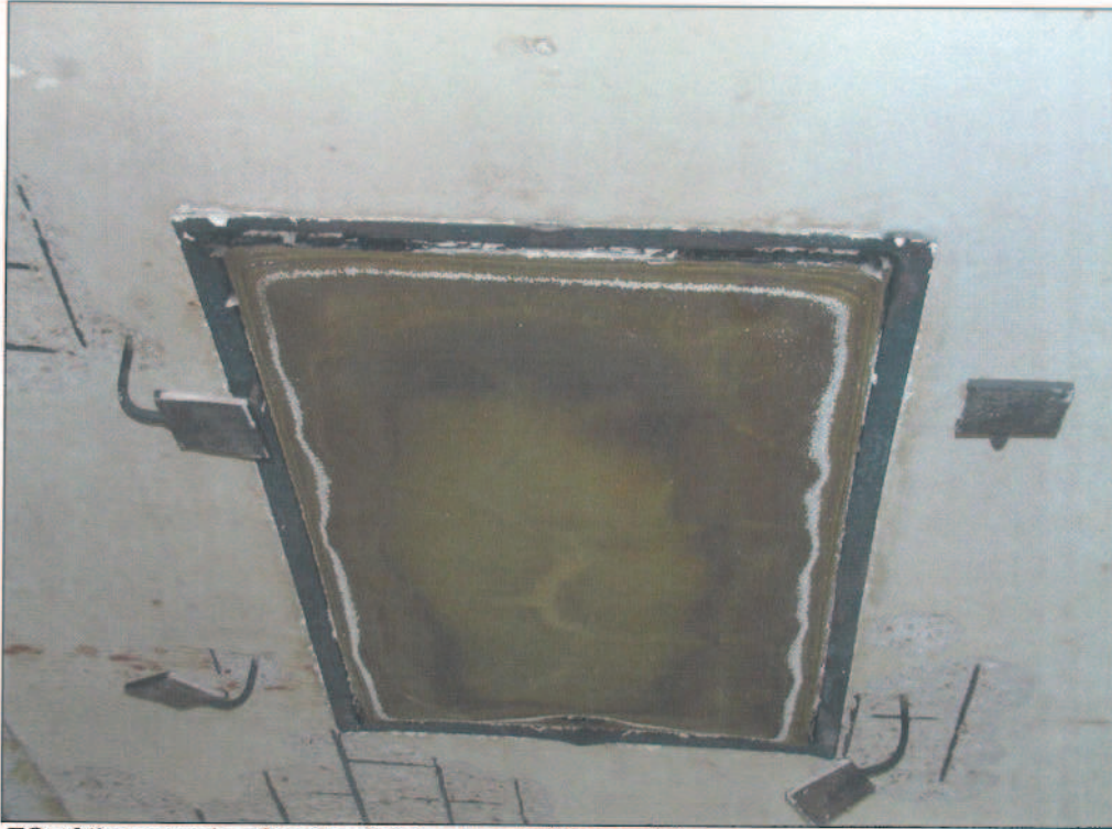
ES of the sample after the finished test of fire resistance
