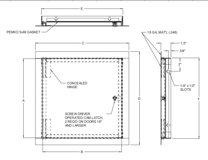
STANDARD FEATURES: SCREW DRIVER OPERATED CAM LATCH,
