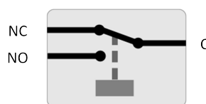
Relay configuration (not energised).
