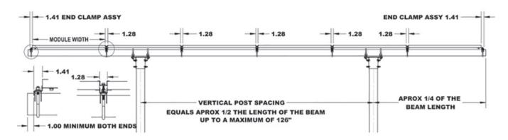
When using a single vertical pole (4" Sch-40 pipe) (1-4 modules) center the beam over the vertical post.
