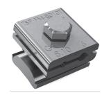
**Ground Lug** Use one per module column to ground rail with bare 6 to 10 AWG copper wire. 88504 8-Pack
