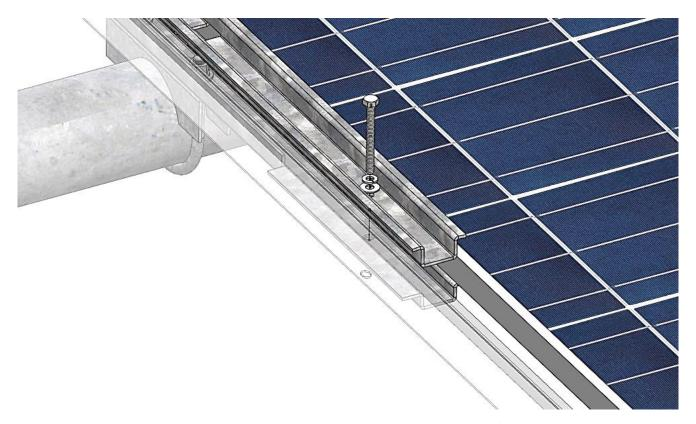
M. Repeat until last module is ready, then add the last end clamp base 1/4" wider than the module width, place the module onto the clamps, center the module, move end clamp base up against the module, attach last mid clamp top and under module clamps as done in previous steps.
