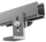
**Rail Mount and L-Foot** Quickly and securely mount the rail from either side, to Tamarack composition shingle flashings, S-5! metal roof clamps or any roof attachment that can be used with a 5/16 inch bolt. **4 mounts and L-feet included.**
