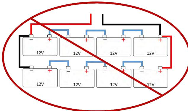
**Do NOT reverse polarity of batteries!**
