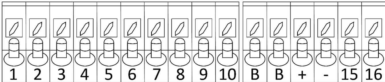
**(1,2) Batt Temp:** Batt Temp Sensor has no polarity; used for voltage correction when using lead acid batteries
