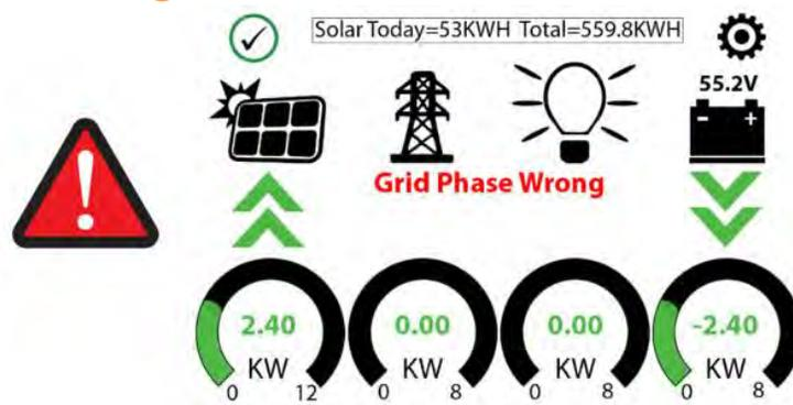
If the Sol-Ark screen shows **Grid Phase Wrong**, there is a phasing issue with your wiring, and it may cause overload faults (F18, F26, F34) even with the Load breaker **off** and **WILL CAUSE DAMAGE if left unchecked**.
