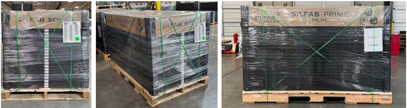
Fig. 7 Horizontal packaging of photovoltaic modules.
