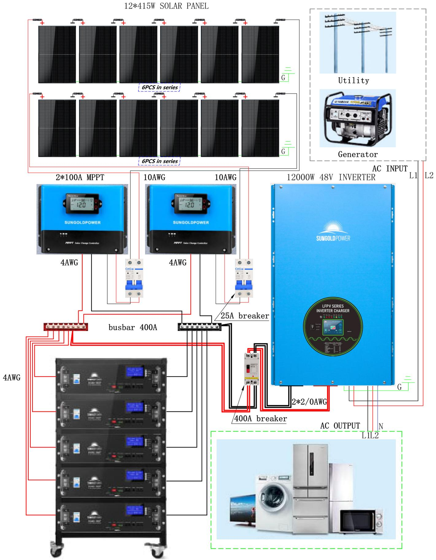
5\*100AH 48V LIFEP04 BATTERY *in parallel*
