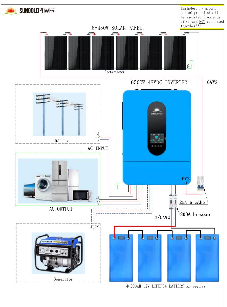
COMPLETE OFF GRID SOLAR KIT 6500W 48V 120V/240V OUTPUT 10. 24KWH LITHIUM BATTERY 2700 WATT SOLAR PANEL
