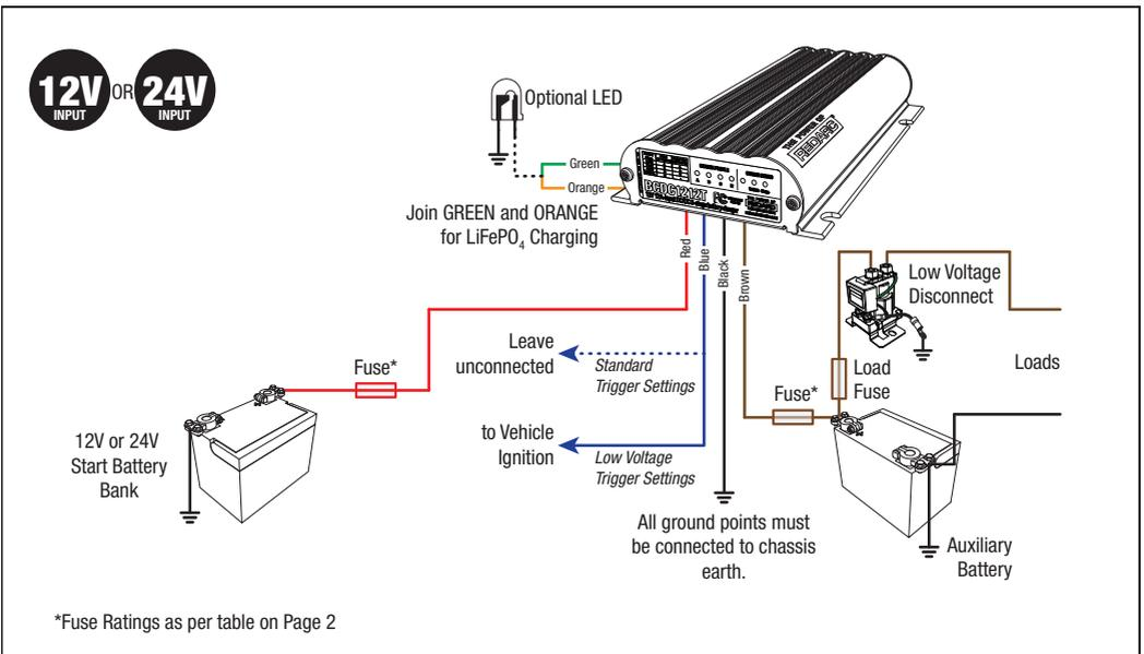
Figure 2.7.2 - Typical LiFePO<sub>4</sub> Setup
