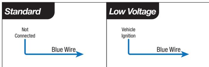
Figure 2.3.1 - Setting the Input Trigger Settings
