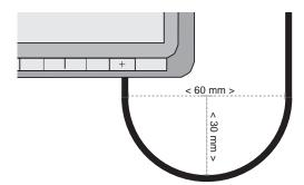
Fig. 9: Minimum bend radius of 30 mm and cable exiting the junction box
