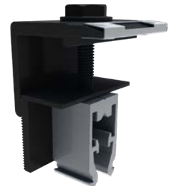
Image 2.4.10-1 Universal end clamp w/WEEB-BMC [96 in-lbs (11 N-m)]
