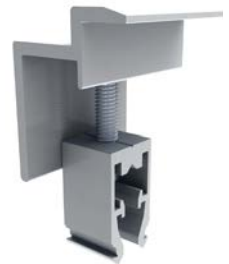
Image 2.4.8 Fixed end clamp [96 in-lbs(11 N-m)]
