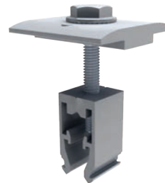
Image 2.4.7 Bonding plate mid clamp [144 in-lbs (16 N-m)]
