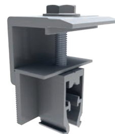
Image 2.4.9 Universal end clamp [96 in-lbs (11 N-m)]
