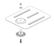
Kit includes flashing, puck, 5/16-inch bolt and nut, o-ring and sealing washer.
