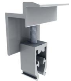
Image 2.4.8 Fixed end clamp [96 in-lbs(11 N-m)]
