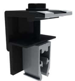
Image 2.4.10-1 Universal end clamp w/WEEB-BMC [96 in-lbs (11 N-m)]
