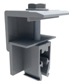
Image 2.4.9 Universal end clamp [96 in-lbs (11 N-m)]
