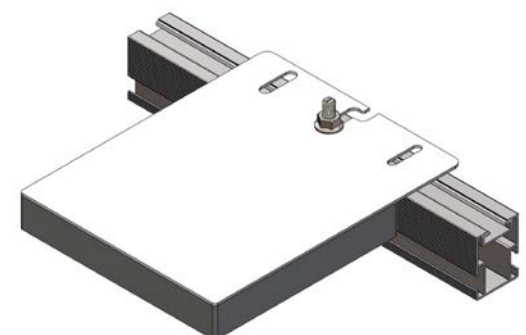
Image 2.4.15 MLPE mounted to QRail with T-bolt.
