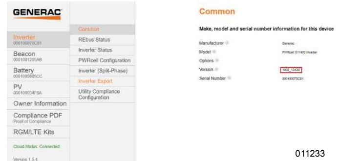
Figure 6-27. Verifying Inverter Firmware
