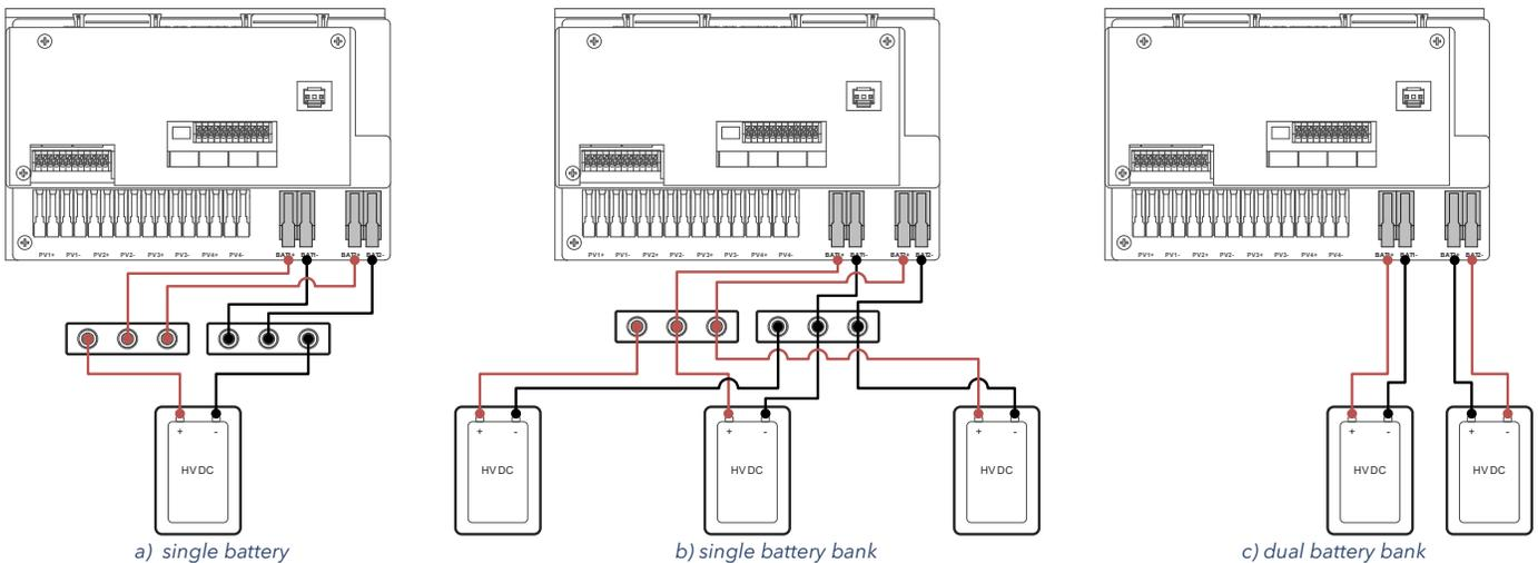
! If a single battery is capable of charging / discharging above 50A, connect the battery to both input terminals. Otherwise, the charge and discharge rate will be limited to 50A max. Connect batteries of the same brand, model, and chemistry to the terminals
