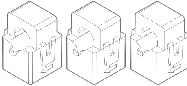
! Off-Grid system do not require CT sensors unless "Grid Peak-Shaving" is used
