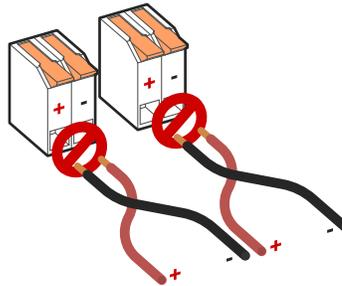
⚠ **DO NOT** reverse polarity. The system will be damaged, and warranty will be voided!
