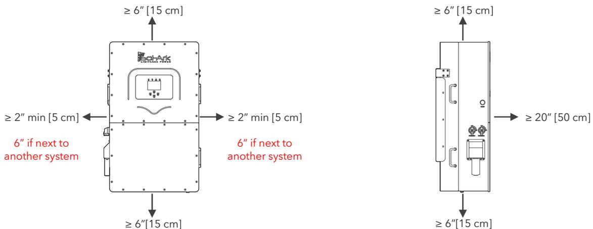
! Max heat dissipation of 1,050W
