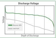
Partial State of Charge (SOC) Discover AES batteries will not suffer negative effects from partial SOC.
