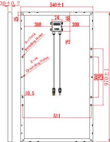
Frame thickness:  $0.9\pm0.12MM$ Treatment for frame: Anodized.
